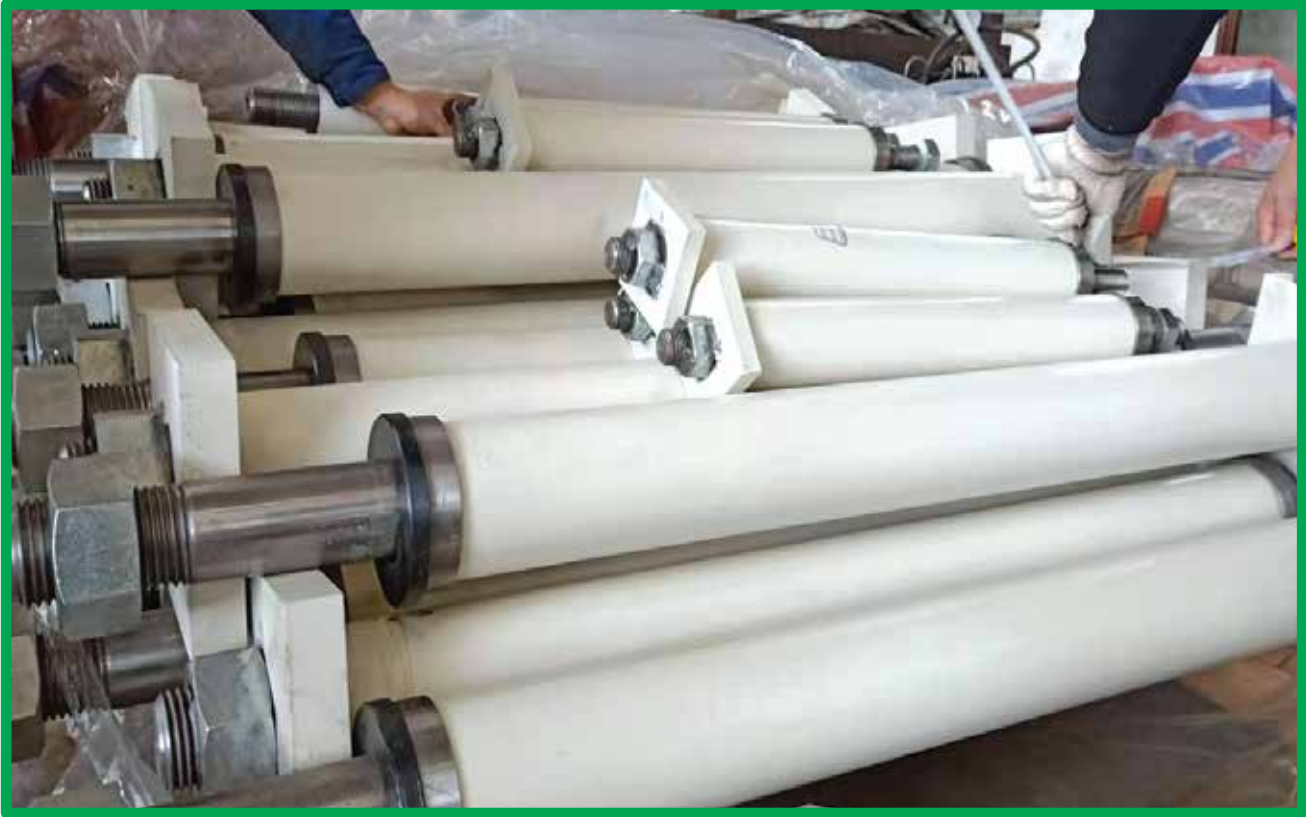
Base Plate and Anchor Bolts of Generator Manufacturing at Factory, China
