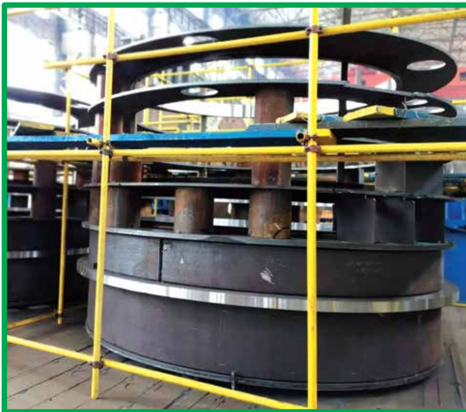
Manufacturing of Frame of the Generator at Manufacturing Facility at China
