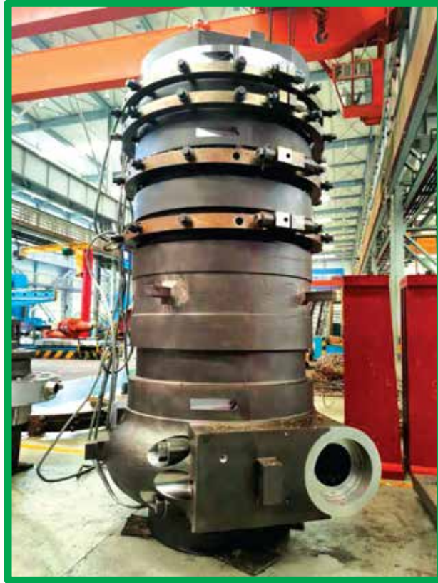
HP Interior Cylinder of Turbine Unit 1 at Manufacturing Facility at China
