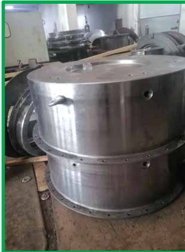
Bearing Box of the #1 Boiler Manufacturing at Factory, China
