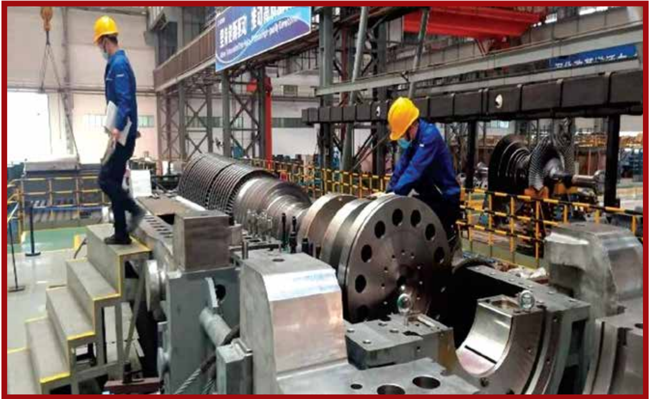
Steam Turbine (Rotor)
