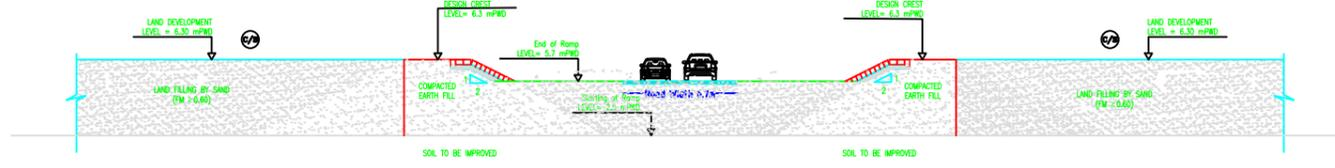
**TYPICAL CROSS SECTION OF EMBANKMENT AT END OF RAMP**
