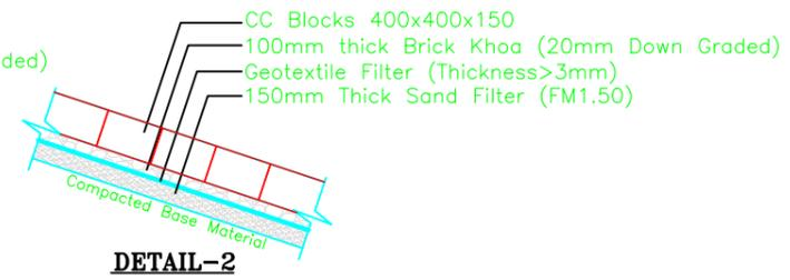
**TYPICAL SECTION OF EMBANKMENT AT START, MIDDLE & END OF RAMP**
